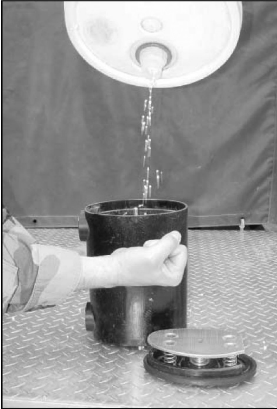
Figure 11-5. Filling canister with absorbent
