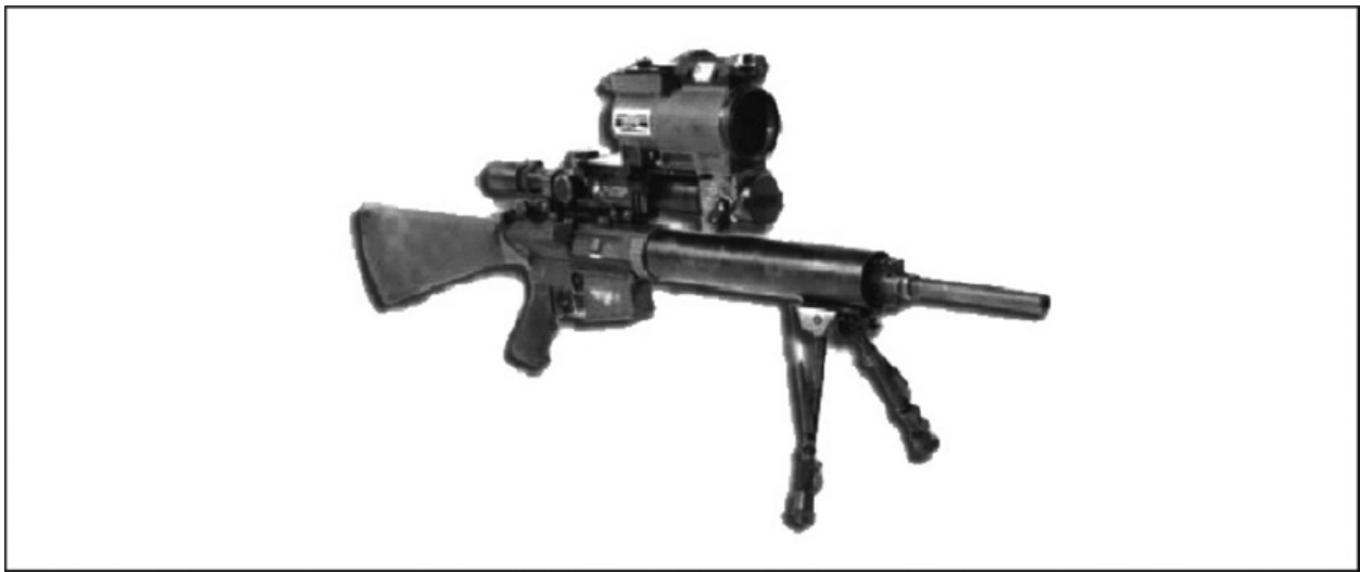
Figure 2-17. NADS 750 with AN/PEQ 2 IR pointer/illuminator mounted on SR-25
