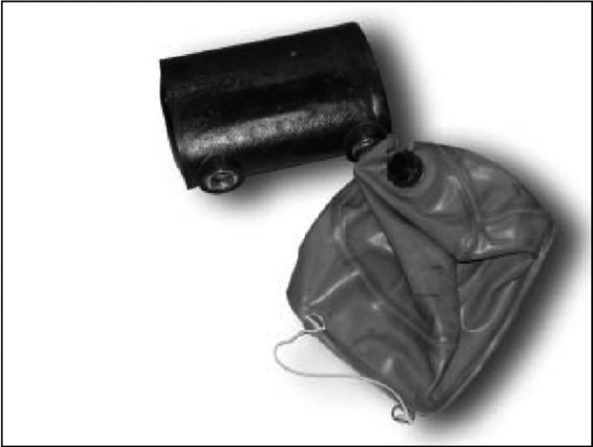
Figure 11-7. Breathing bag attached to scrubber canister
