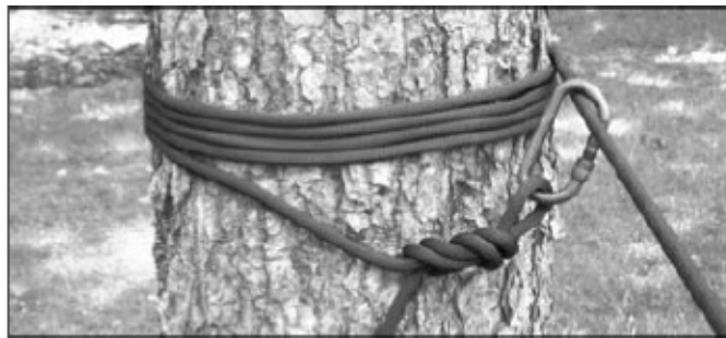
Figure 5-4. Tensionless natural anchor
