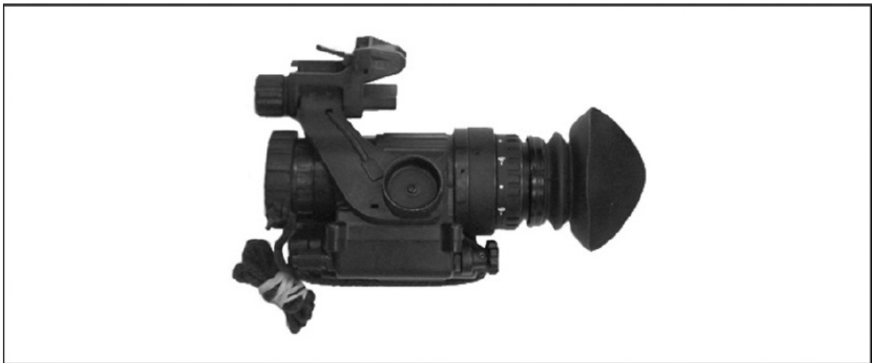
Figure 2-25. AN/PVS-14 Mounted with helmet clip
