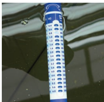
Measure the starting EC after adding water to the reservoir.
