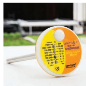
DLI meter that measures total light delivered in 24 hours using \text{mol}/\text{m}^2/\text{day}
