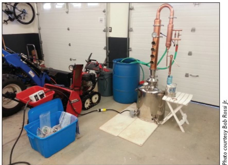
A flute distiller on a 26-gallon keg, heated with an electric kettle.
