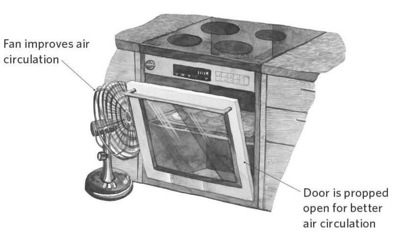
To use an oven to dehydrate food, you must be able to set the oven for 140°F to 170°F (60°C to 80°C). At higher temperatures, the food cooks rather than dries. Your drying racks should be 3 to 4 inches shorter than the oven from front to back. Wire cooling racks placed on top of cookie sheets work well for some foods. Set the oven racks that hold the trays 2 to 3 inches apart for good air circulation.
