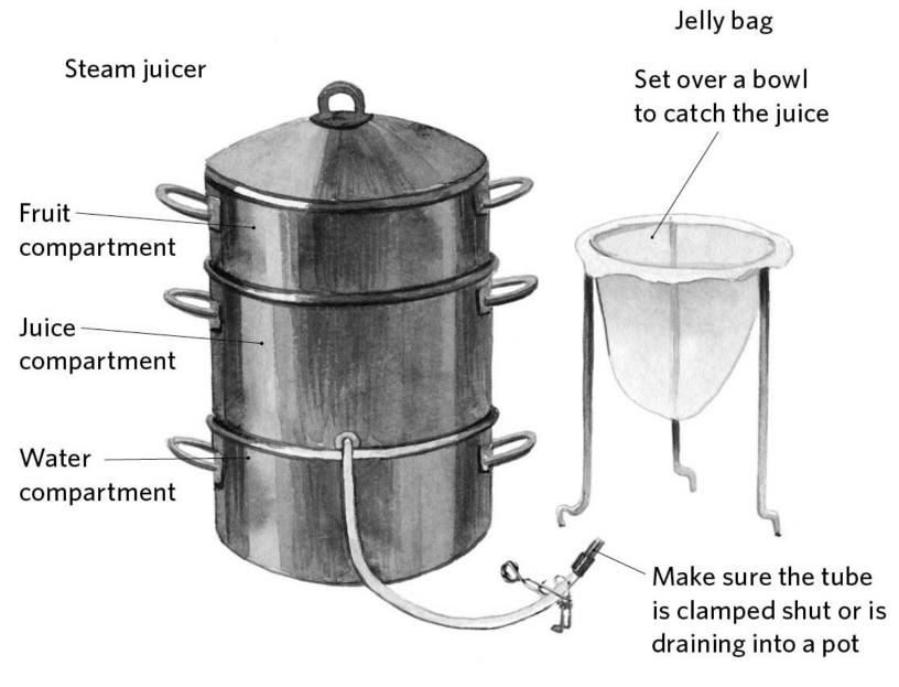
ABOVE: The steam juicer works to cook the fruit and separate the fruit from the juice. With a jelly bag, you must cook the fruit on the stove, then pour it into the jelly bag to drain.
