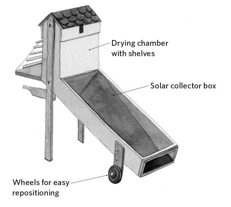
A solar dryer has three basic parts: a solar collector (such as an old storm window), a box to hold the food, and a stand. The collector captures the heat of the sun to warm air that will circulate around the food. The box is usually made from plywood and holds food trays, which are made from screening to allow greatest air circulation. The most sophisticated solar designs include adjustable vents and thermostats.
